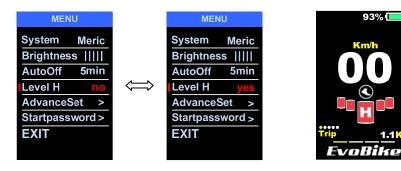
**8.5 Advance setting**: Press POWER button can get into the advance setting menu, default password is '1919'.
