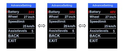
**8.9** Wheel: Press UP/DOWN can change the wheel setting, optional wheel diameter is 10 ~ 30 inch.
